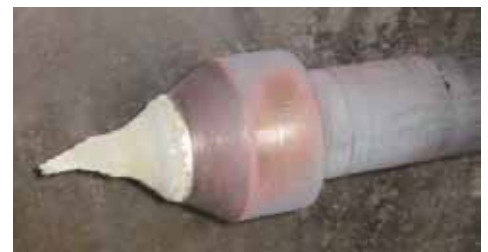
Varying levels of stem plug wear (depending on the application or how abrasive the fluids are, internals may wear faster).
