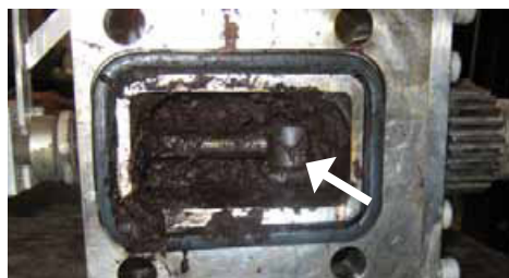
Left to right: foreign objects may flow into the combining tube, cause damage and render the heater inefficient; disassembling the heater will show hidden build-up that hinders operation (pictured: starch build-up in the CTA has hardened and stopped rotation); internals may snap (pictured: retaining ring) and cause nozzle vibration which will result in damage to the body.
