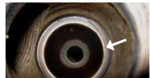
Left to right: foreign objects may flow into the combining tube, cause damage and render the heater inefficient; disassembling the heater will show hidden build-up that hinders operation (pictured: starch build-up in the CTA has hardened and stopped rotation); internals may snap (pictured: retaining ring) and cause nozzle vibration which will result in damage to the body.
