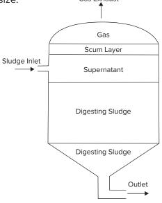
heat the combined inflow and circulation streams to the desired temperature. In either case, the digester temperature can be maintained precisely (+/- 1°F or 0.5°C) with adequate instrumentation, allowing the digestion process to be fine-tuned for optimum results.
