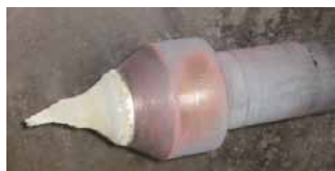
Stem plug wear: depending on the application or how abrasive the fluids are, internals may wear faster.
