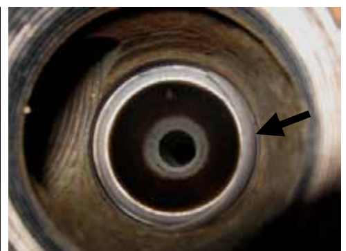
Stem plug wear: depending on the application or how abrasive the fluids are, internals may wear faster.
